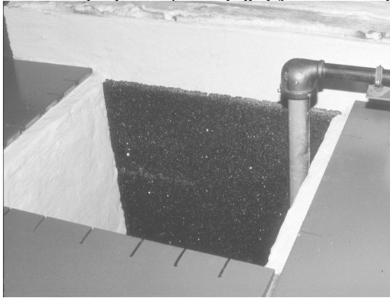
Figure 1a: Vertical Gate Filters are placed in the outlet well or dipwell of a casting furnace.
