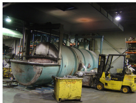
Fig. 4. The 10,000-kg barrel furnace.
